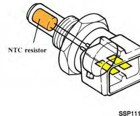
A coolant temperature sensor is located at the back of the cylinder head. It is an NTC resistor.
