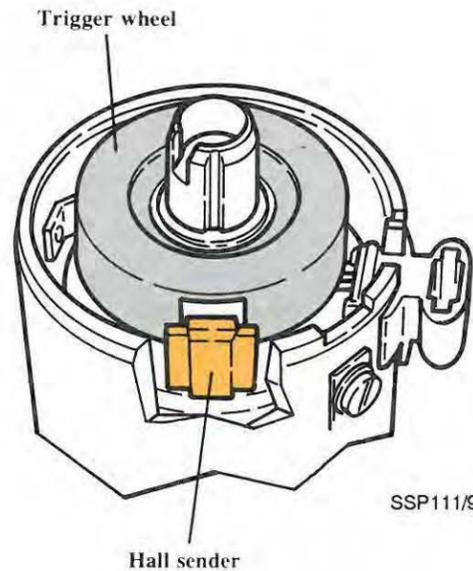
The Hall sender and trigger wheel are located in the distributor. The trigger wheel has a 40° wide opening (Hall window).
