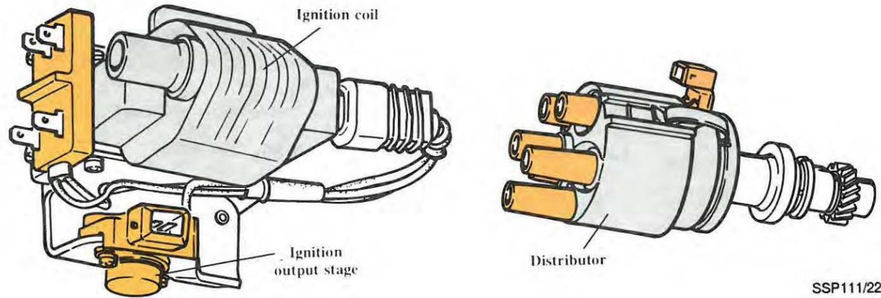
An ignition coil with a separate power stage is used with the Motronic system. The power stage is a Darlington-type of transistor which switches the primary current for the ignition coil on and off.
