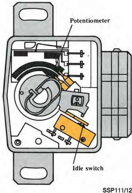
An idle switch and throttle valve potentiometer are used on the throttle assembly. The idle switch closes at approximately  $1.3^\circ$  before the throttle plate closes. When the switch is closed, this signal is used to activate the following functions:
