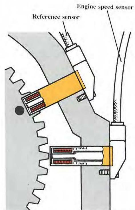
Both sensors are identical in design and are located on the left side of the engine compartment, near the flywheel.
