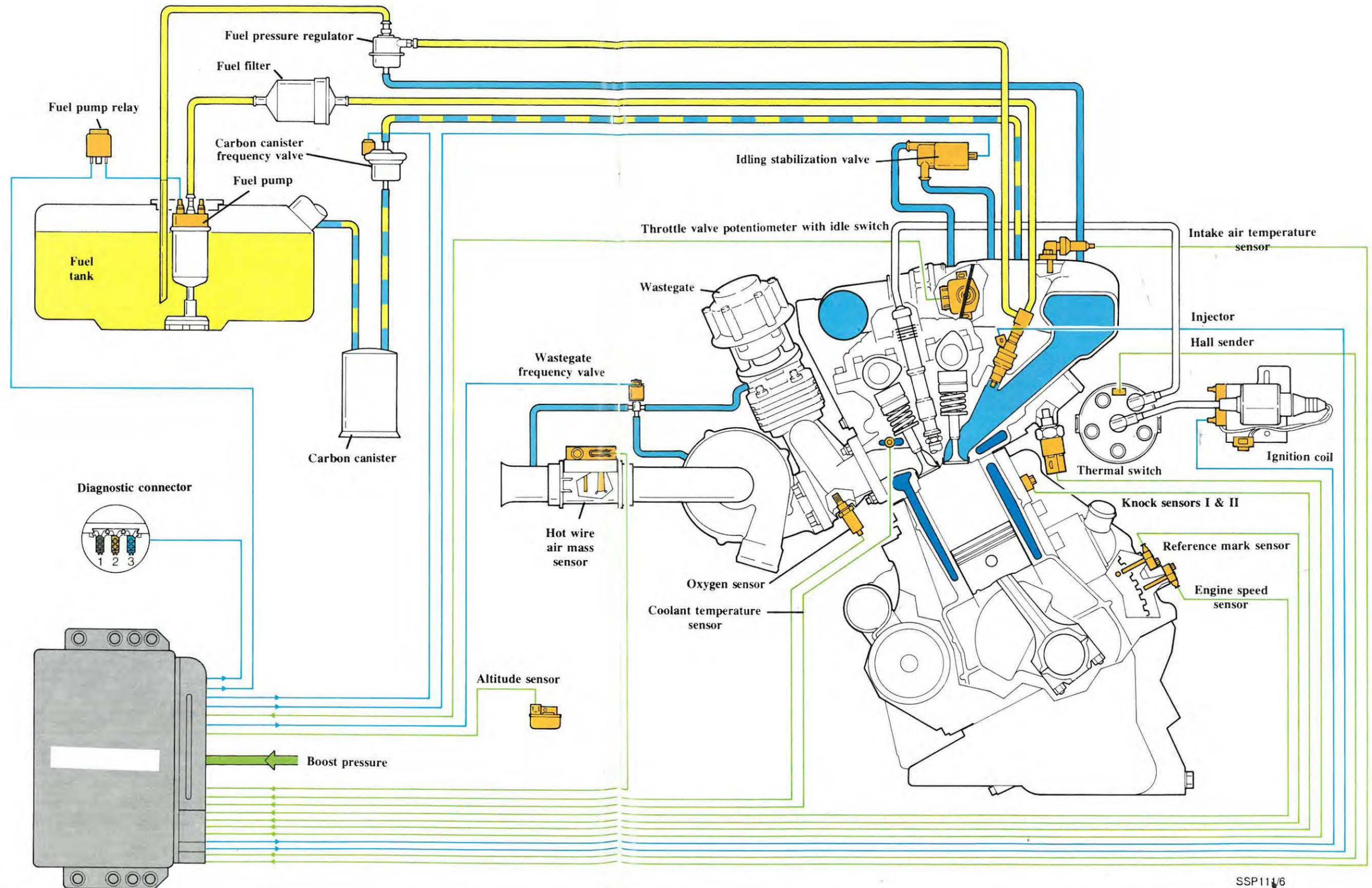
The Motronic control unit performs the following functions:
