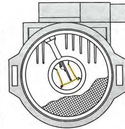
A hot wire air mass sensor is located ahead of the turbocharger and is mounted to the air filter housing. The sensor is used to measure the air flow into the engine. The sensor uses a glass-coated, thin platinum wire to measure the air flow, and contains no moving parts.
