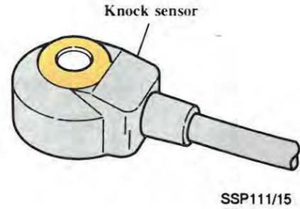
The 20-Valve turbo uses two knock sensors. Knock sensor I is located next to cylinder #2 and is used for cylinders #1, #2 and #3. Knock sensor II is located next to cylinder #4 and is used for cylinders #4 and #5.
