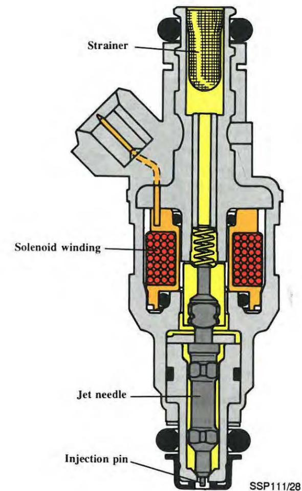
The housing contains the solenoid winding and the guide for the needle jet. When a ground is supplied to the solenoid winding, the needle jet is pulled away from the seat and the pressurized fuel exits the injector.
