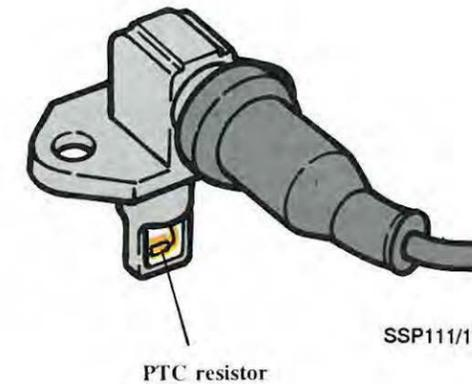
An intake air temperature sensor is located in the intake manifold near the throttle valve housing. It is used for ignition timing, knock regulation and boost pressure control. The sensor is a PTC resistor.
